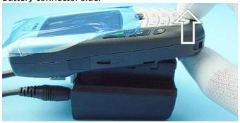
When removing the Flash Adapter, always start from the bottom side of the unit.
