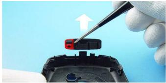
The Power Button can be removed easily.
