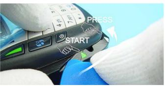
Place the SRT-6 on the Jig and shift it carefully along the edge of the Jig. Start at green mark to release the A-Cover, use it like a blade with moderate force only, to prevent damages at the covers. Shift the SRT-6 to the next mark and carefully press in the tip. (watch videos)
