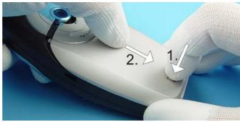
Press the Release Button before removing the C-Cover.
