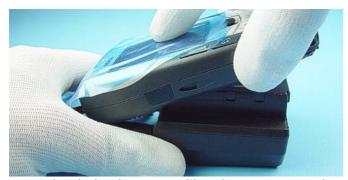
Insert the Flash Adapter SF-2 like a battery, start at the Battery Connector side.
