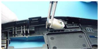
Use tweezers when removing the Vibra Motor.
