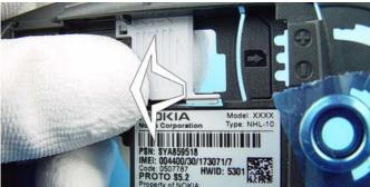
To remove Locking Lever place it in the shown position first, than push it from the other side with moderate force.
