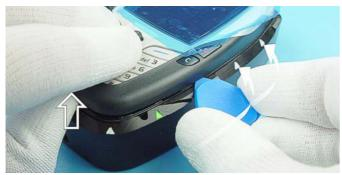
Lift the A-Cover on its bottom side carefully. Place the SRT-6 in the groove and shift it to the next mark. Then press in the tip as in the step above.
