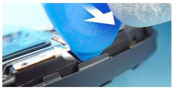
Use the SRT-6 as a lever to release the snap. Do not twist SRT-6, because this would damage the cover.
