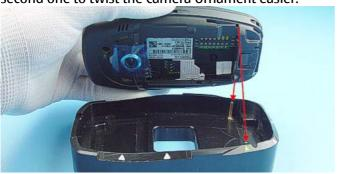
Place the unit into the Disassembly Jig SS-12. Note that guiding pins are positioned correctly into the gaps.
