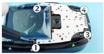
Unscrew the four Torx Plus® size 6 screws using the order shown. For assembly, the reverse order and a Torx Plus® driver with a torque of 19Ncm have to be used.
