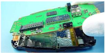
Now, the Engine Module can be removed.
