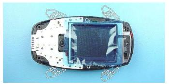
The UI Support Frame is attached with four snaps in B-Cover.
