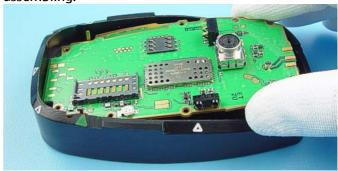
To prevent damages of spring contacts use always the disassembly jig when removing VGA Camera.
