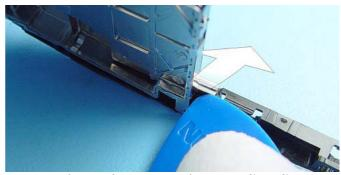
SRT-6 can be used to remove the Grounding Clip.
