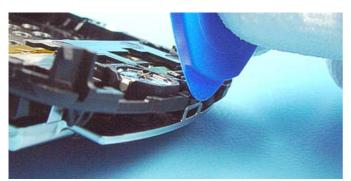
Release the next snap by using the SRT-6.
