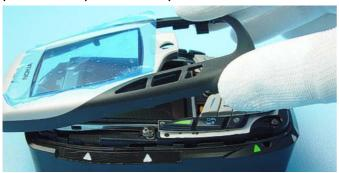
Now, the A-Cover can be pulled up. Always protect the inner side of the window and LCD with a film.
